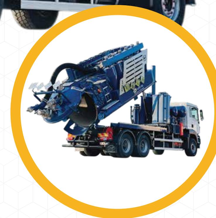
The IVT SUPERVAC industrial vacuum loader with cyclone separator is designed for heavy industrial applications and is suitable for suctioning, displacing (option), transporting and discharging dry, wet and hazardous substances, such as various types of catalyst, gravel, powders, fly ash and sludge. Specially developed for working with hazardous and contaminated substances, the system is available in ADR / API versions and built-in accordance with all applicable safety standards.
