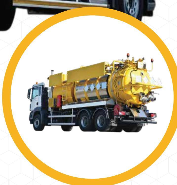
The POWERVAC X is specifically designed for suction, transporting, and unloading of liquid and hazardous substances such as liquids, sludge, fats, oils, fuels, and chemicals in the (heavy) industry. This robust machine operates gently with a 3400m<sup>3</sup>/h liquid ring vacuum pump. Specially developed for working with hazardous and contaminated substances, the truck is available in ADR / API2219 versions and built in accordance with all applicable safety standards.
